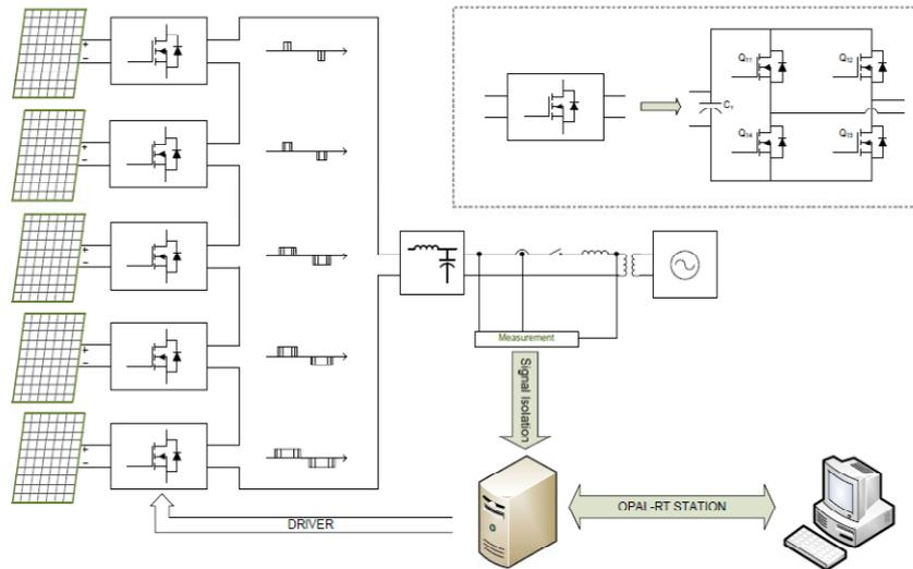
Figure 2. Multilevel inverter system overview
