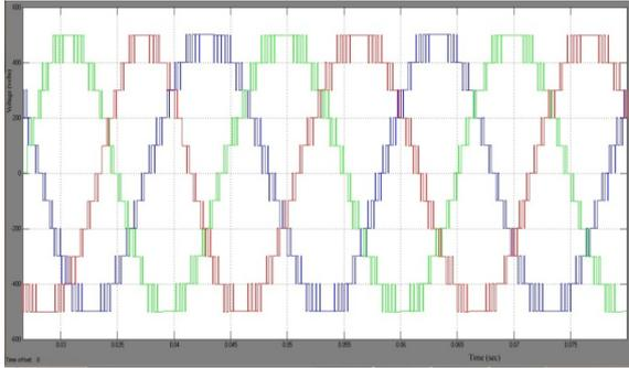
Figure 3(a). Grid Voltage without PV cell
