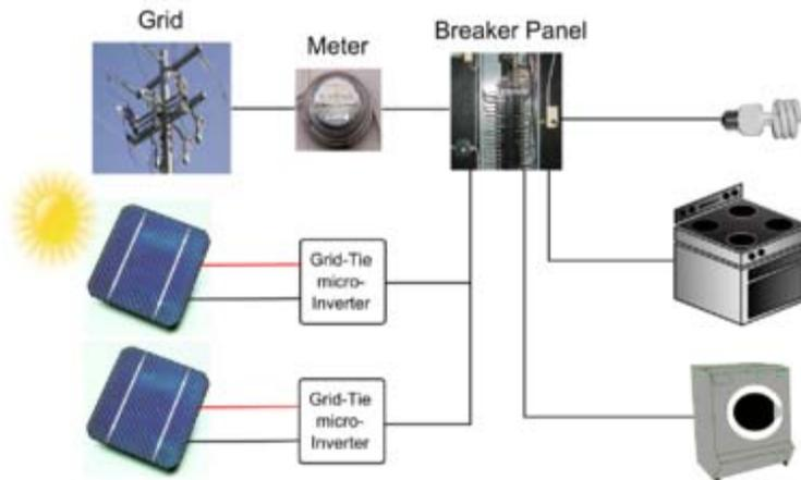
Figure 1. Diagram of a residential grid-connected PV system
